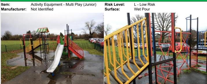
**Finding:** The unit is easily accessible and has an opening in **Action:** Monitor - No action given the risk assessment the barrier to steep play elements in excess of 500mm in contravention of BS EN 1176 Part 1
