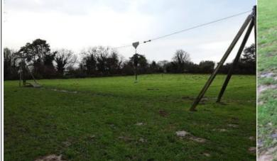
**Finding:** The grass mats are silted up and the soil is compacted; this may have an effect on the impact absorbing properties of the surface. Consideration should be given to HIC testing the surface to verify impact attenuating properties ( https://playinspections.co.uk/inspectionservices/safety-surface-testing/ )
