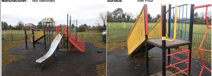
**Finding:** The unit is easily accessible and has an opening in **Action:** Monitor - No remedial work recommended the barrier to steep play elements in excess of 500mm in contravention of BS EN 1176 Part 1
